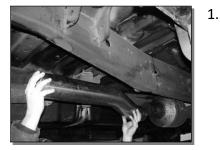
Install the Extension Pipe over the catalytic converter. See Figure 2. The Extension Pipe provided is pre-cut for the crew cab long bed configuration. All other configurations will require this pipe to be cut. Extended cab short bed cut to 15 3/4" Crew cab short bed cut to 29" Extended cab long bed cut to 31"
