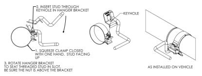
4. Install the 18" Extension Pipe over the Mid Pipe. The 34" Extension Pipe is pre-cut to fit vehicles with a 172" wheelbase and will have to be cut to fit all other vehicles. 137" wheelbase vehicles do not require the 34" Extension Pipe to be installed. The Hang Tight<sup>™</sup> Hanger Clamp Assembly is used at the connection between the 18" Extension Pipe and the 34" Extension Pipe and the 34" Extension Pipe and is installed into the OEM rubber hanger at this position.
