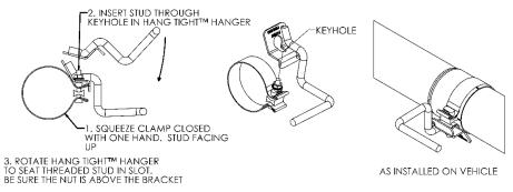
Figure 6 (Hang Tight<sup>TM</sup> Hanger not exactly as shown).
