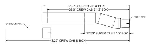
4. Install the **Front Pipe** to the vehicle using the **3" Clamp** provided. Place the **Hang Tight<sup>TM</sup> Hanger** into the existing rubber isolator. Install the **Extension Pipe** to the **Front Pipe** if required. **Refer to Figure 3.**
