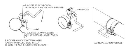
4. Install the hanger assembly from step 3 loosely to the **Extension Pipe** (or **Front Pipe** if the **Extension Pipe** is not required) and place the hanger into the existing rubber insulator. **Refer to Figure 5.**
