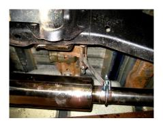
3. Install the **Muffler** onto the **Extension Pipe** using the **Hang Tight**<sup>TM</sup> **Hanger Clamp Assembly**. Then install the **Hang Tight**<sup>TM</sup> **Hanger** into the factory rubber insulator. Do not tighten the clamp at this time. **Refer to Figure 5**.
