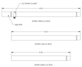
3. Using the **3" Clamps**, install the **Muffler** onto the **Extension Pipe** (or **Mid Pipe** if required), and install the **Over Axle Pipe** into the opposite end of the **Muffler**. Install the **Over Axle Pipe** hanger into the factory rubber insulator located above the rear of the **Muffler**.
