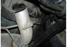
1. Apply a penetrating lubricant liberally to all exhaust fasteners, hangers and rubber insulators.
