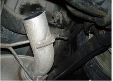
2. The tail pipe will need to be cut to clear the rear axle. Refer to Figures 1&2.
