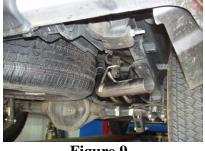
8. Slide a 2 ½" Clamp onto the Driver Side Tail Pipe then attach to the Driver Side Over Axle Pipe. Using fasteners provided attach the Hanger Assembly to the bottom of the frame. Refer to Figure 10.
