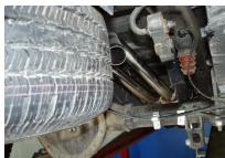
5. Slide a 2 ½" Clamp onto the Passenger Side Over Axle Pipe and slide onto the passenger side of the Muffler. Attach the hanger to the factory rubber insulator. Refer to Figure 8.
