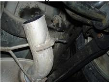
Pamova the hangers from the rubber insulators and remove the exhaus
