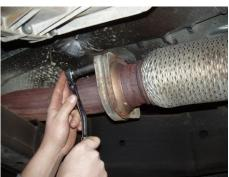
3. Remove the hardware holding the front flange together and disconnect exhaust system. **Refer to Figure 3**.
