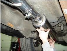
5. Install and adjust the **Exhaust Tip** to suit. Use a 17mm wrench to tighten the lock bolt located on the **Exhaust Tip**.
