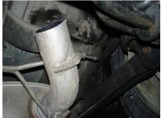
1. Apply a penetrating lubricant liberally to all exhaust fasteners, hangers and rubber insulators.
