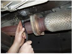
3. Remove the hardware holding the front flange together and disconnect exhaust system. Refer to Figure 3.
