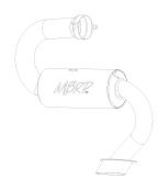
NOTE: To avoid exhaust leaks use high heat silicone to seal all connections between expansion chambers and muffler. Monitor for leaks during the first 200 miles after your installation and re-apply silicone where necessary. We suggest having your local snowmobile mechanic or performance shop install this product.
